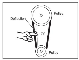
Figure 69. Checking V-belt tension.
